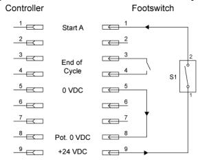
— Connections on pin 3 and 4 have to be made seperately!
