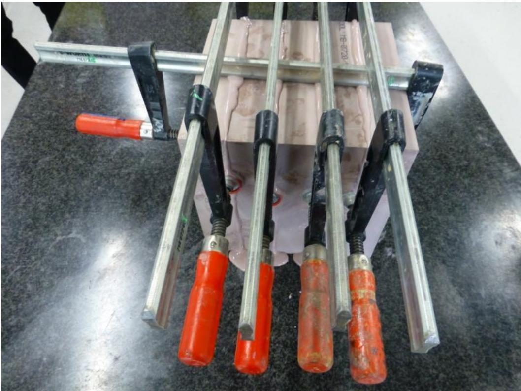
Apply clamping pressure (e.g. vise) to the parts/casting to be bonded until the excess adhesive is pushed out, then reduce pressure and leave to cure.
